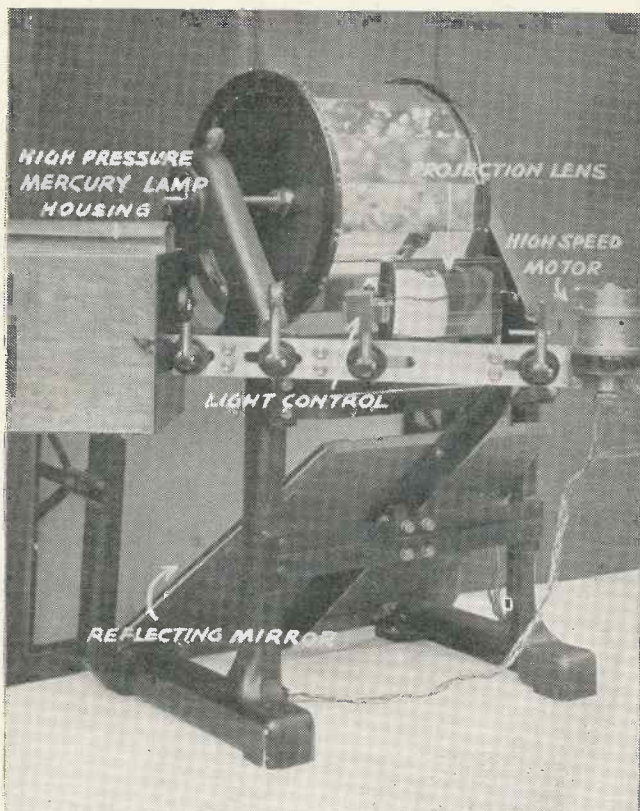
Rear view of the Scophony receiver showing the optical arrangements and light control.
